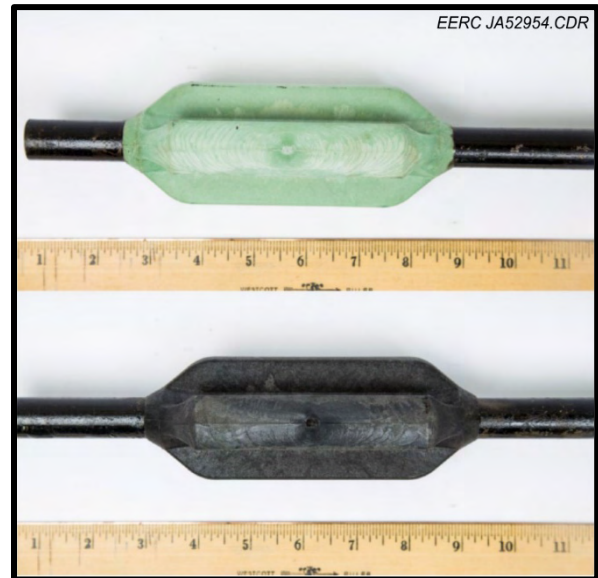
Figure 21. Types of sucker rod guides analyzed.
