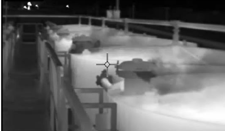
Infrared video image of thief hatch emissions. U.S. EPA, 2015.
